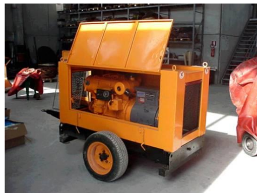
Rotative Motorwelding 400 A output Motosaldatrice rotativa da 400 A
