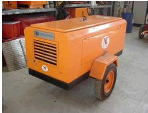
Rotative Motorwelding 300 A output Motosaldatrice rotativa da 300A
